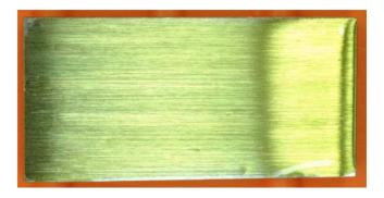
Test with Ferroxyl Solution applied to one of its surfaces after 4 minutes of testing. No indications of iron/iron oxide particles.
